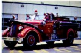
1957 Seagrave Quint 750 GPM/75' aerial ladder First such apparatus in Kentucky! 1957-1986
